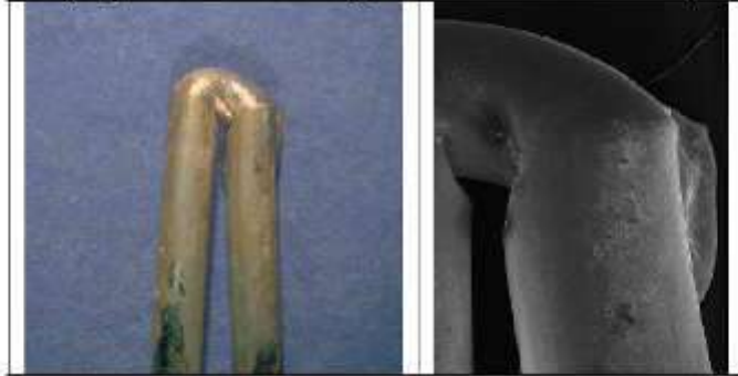
Figure 2 Overview photograph and SEM image of conductors fused by arcing through char.
